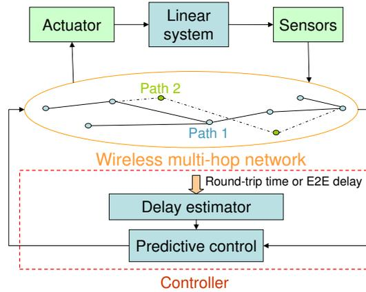
**Fig. 6.1** Overview of the system and control setup.
