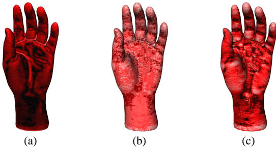
Fig. 11 Several curvature estimations on the hand model: mean curvature (a), Gaussian curvature (b) and curvature index (c) [19]. The curvature index generates a more important contrast between convex and concave areas.
