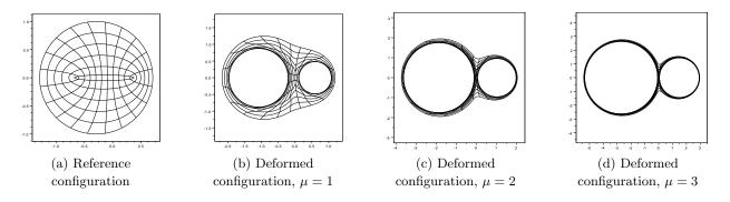
Figure 3: Incompressible deformation of  $B(\mathbf{0}, d)$ ,  $d := |\mathbf{a}_2 - \mathbf{a}_1|$ , for increasing values of  $\mu := \sqrt{\frac{v_1 + v_2}{\pi d^2}}$ . Final cavity volumes  $v_1$  and  $v_2$  given by d = 1,  $\frac{v_2}{v_1} = 0.3$ .
