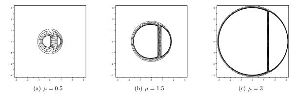
Figure 2: Incompressible deformation  $\mathbf{u} : B(\mathbf{0}, d) \setminus \{\mathbf{a}_1, \mathbf{a}_2\} \to \mathbb{R}^2, d = |\mathbf{a}_2 - \mathbf{a}_1|$ , opening distorted cavities of volumes  $v_1 + \pi \varepsilon_1^2, v_2 + \pi \varepsilon_2^2$ ; deformed configuration for increasing values of the displacement load ( $\mu := \sqrt{\frac{v_1 + v_2}{\pi d^2}}$ ). Choice of parameters:  $d = 1, \frac{v_2}{v_1} = 0.3$ .
