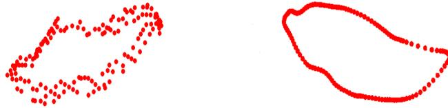
**Fig. 3** Left: extracted level set on an irregular mesh. Right: an extracted level set on the regular mesh after refinement.
