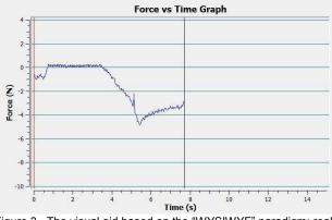
Figure 3. The visual aid based on the "WYSIWYF" paradigm: realtime plot of the force applied by the needle vs. the time
