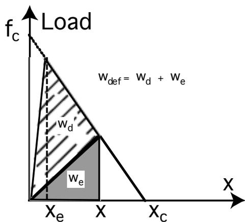
Figure 7 : Energy balance at elongation  $x$
