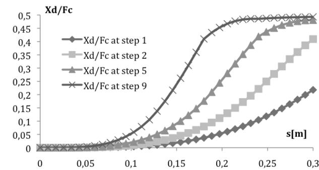
Figure 18 : Evolution of  $f_x$  along the beam
