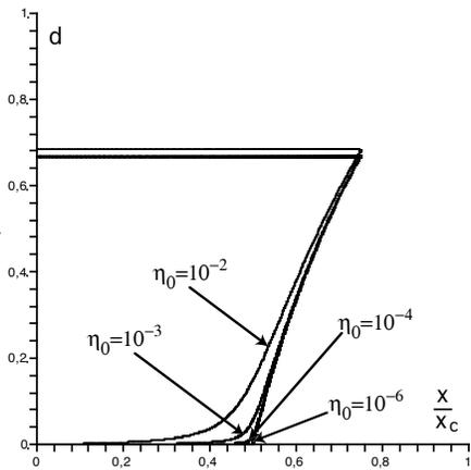
Figure 5: Influence of  $\eta_0$  on damage variable
