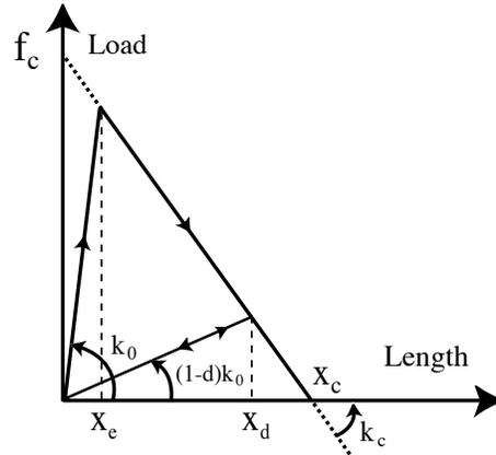
Figure 1: The “triangle” damageable elastic interface behaviour
