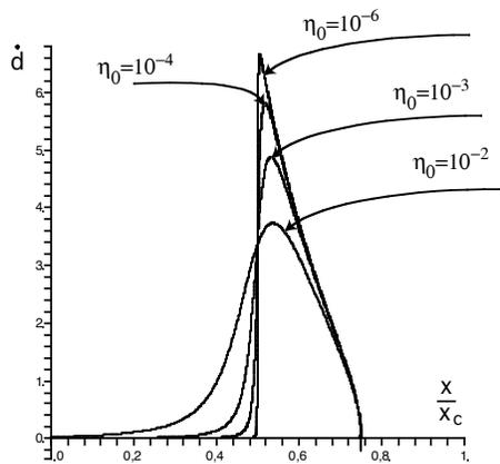
Figure 6 : Influence of  $\eta_0$  on damage rate evolution
