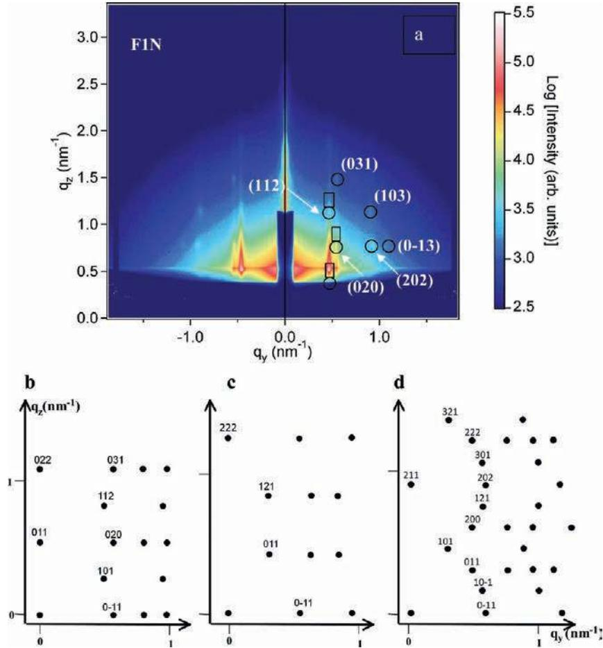
**Figure 5.** (a) GISAXS pattern of the F1N sample (cubic indexation). (b–d) GISAXS pattern schemes for the Im-3m structure according to orientations with different directions perpendicular to the substrate: (b) [011] direction;<sup>43</sup> (c) [111] direction;<sup>43</sup> (d) [211] direction. Patterns have been simulated with a cubic unit cell at 16 nm.
