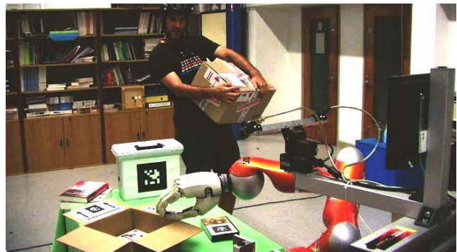
Fig. 1 Interacting with the robot in an everyday setup: the human asks for help in vague terms, the robot takes into account the human’s spatial perspective to refine its understanding of the question.
