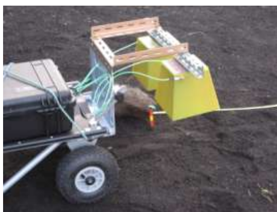
Figure 1 : Experimental set-up for field tests. The electronic unit and the batteries are in the black box. The transmitting and receiving yellow antennas are identical[2]
