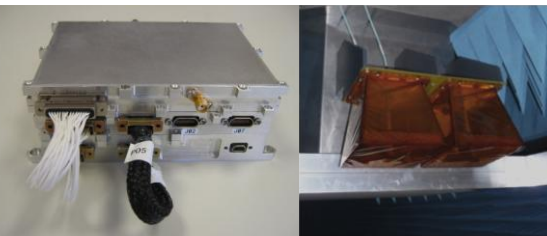
Fig. 2: Electronic Unit (left) and antenna system mounted on a rover mockup (right).
