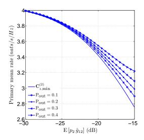
Figure 6. Primary mean rate,  $C_1$ , versus mean interference power,  $\mathbb{E}[p_2 \hat{g}_{12}]$ , for different values of outage probability  $P_{out}$ .
