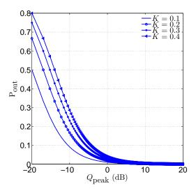
Figure 8. Outage probability,  $P_{out}$ , versus peak interference power,  $Q_{peak}$ , for different values of minimum received power, K, required for secondary service.
