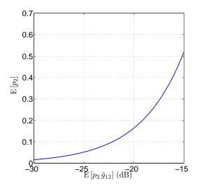
Figure 10. Mean transmit power,  $\mathbb{E}[p_2]$ , versus mean interference power,  $\mathbb{E}[p_2 \hat{g}_{12}]$ , for  $P_{out} = 0.1$ .
