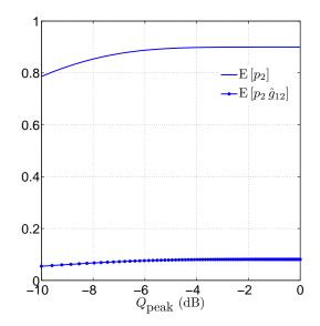
Figure 7. Mean transmit power,  $\mathbb{E}[p_2]$ , and mean interference power,  $\mathbb{E}[p_2 \hat{g}_{12}]$ , versus peak interference power  $Q_{\text{peak}}$ .  $p_{2,\text{peak}} = 1$ and  $P_{\text{out}} = 0.1$ .
