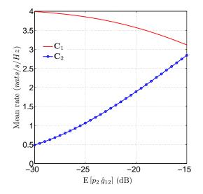
Figure 9. Primary mean rate,  $C_1$ , and secondary zero-outage capacity,  $C_{2,out}$ , versus mean interference power,  $\mathbb{E}[p_2 \hat{g}_{12}]$ , for  $P_{out} = 0.1$ .
