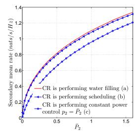
Figure 3. Secondary mean rate versus mean power for different power control schemes: (a) optimal power control *water-filling*; (b) proposed scheduling approximating the optimal power control; (c) constant power control that provides the lower bound of the primary mean rate.  $\bar{P}_1 = 1$ ,  $\sigma^2 = 0.01$  and  $\lambda_{11} = \lambda_{12} = \lambda_{22} = \lambda_{21} = 1$ .
