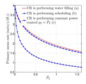
Figure 2. Primary mean rate versus secondary mean power for different power control schemes from the secondary user: (a) optimal power control *water-filling*; (b) proposed scheduling approximating the optimal power control; (c) constant power control that provides the lower bound of the primary mean rate.  $\bar{P}_1 = 1$ ,  $\sigma^2 = 0.01$  and  $\lambda_{11} = \lambda_{12} = \lambda_{22} = \lambda_{21} = 1$ .
