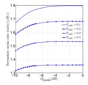
Figure 5. Secondary mean rate,  $C_2$ , versus peak interference power,  $Q_{\text{peak}}$ , for different values of outage probability  $P_{\text{out}}$ .
