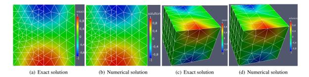
Figure 5. Exact and Numerical solutions in 2D and 3D for mortar method using higher order approximations
