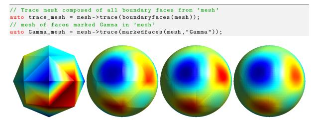
Figure 1. Sphere discretized with 31 elements. Visualization of a function in Gmsh using tetrahedral elements of order N = 1, 2, 3, 4.
