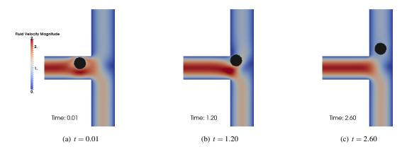
Figure 12. 2D simulation of a particle entering in the low flow rate channel.
