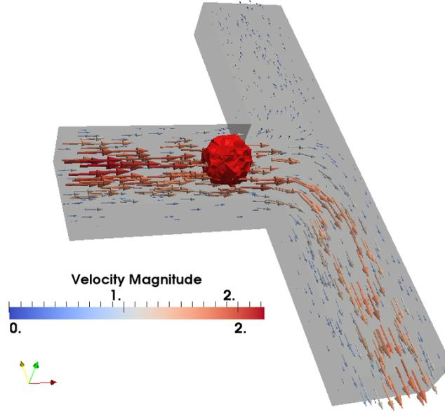
**Figure 13.** 3D simulation of the bifurcation problem. The velocity vectors are plotted and colored by the velocity magnitude.
