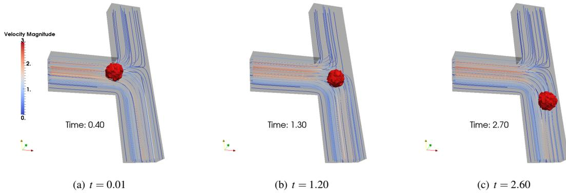
**Figure 14.** 3D simulation of a particle entering in the high flow rate channel. Streamlines are represented and colored by the velocity magnitude.
