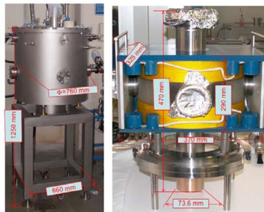
Fig. 1. Photographs of the cryostat (left) and of the 8 T superconducting magnet with its four radial access ports (right).
