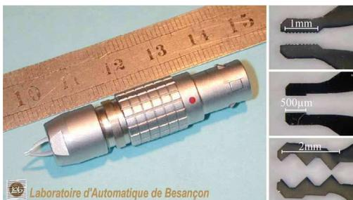
Fig. 2. MMOC Microgripper (left) and finger tips (right).
