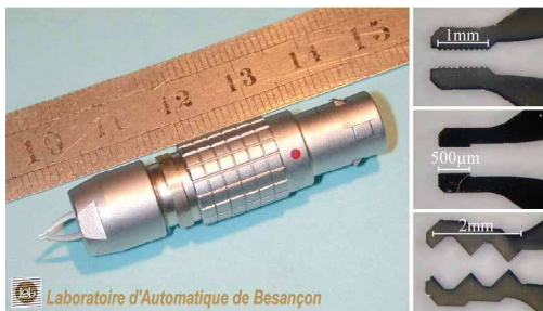
Fig. 2. MMOC Microgripper (left) and finger tips (right).
