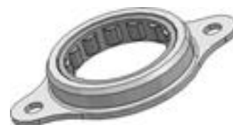
Fig. 2. Example of parametric roller bearing CAD model.
