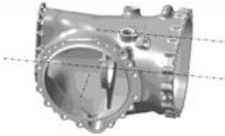
Fig. 5. MGB housing with axes driven by external publications.
