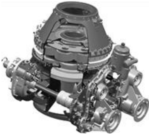
Fig. 1. Example Eurocopter main gearbox CAD Model.
