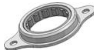
Fig. 2. Example of parametric roller bearing CAD model.
