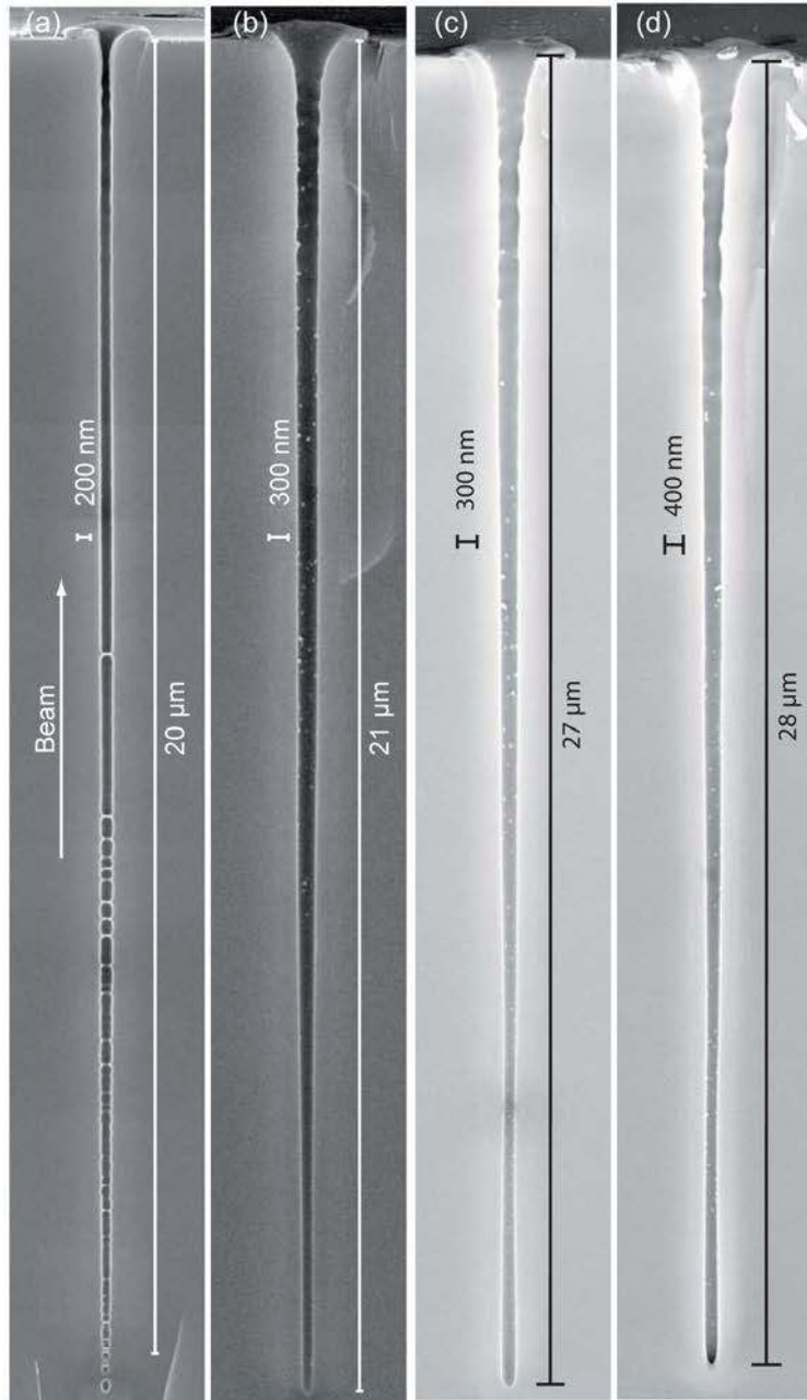
Figure 3 SEM images of cleaved nanochannels processed in glass with single laser shot: (a) \theta=17^\circ, E=0.65\mu\text{J} (b) \theta=17^\circ, E=0.85\mu\text{J} , (c) \theta=11^\circ, E=1.9\mu\text{J} , (d) \theta=11^\circ, E=2.1\mu\text{J}
