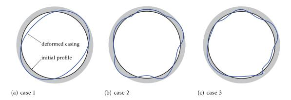
Figure 13: Magnified distortion of the casing
