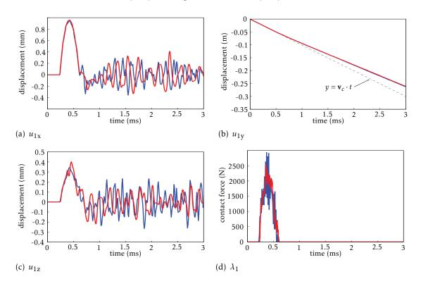
Figure 8: High speed configuration with friction; proposed algorithm (——) and bi-potential method (——)
