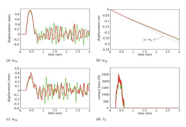
Figure 10: High speed with friction, comparisons between the proposed algorithm (——) and Ansys (——)
