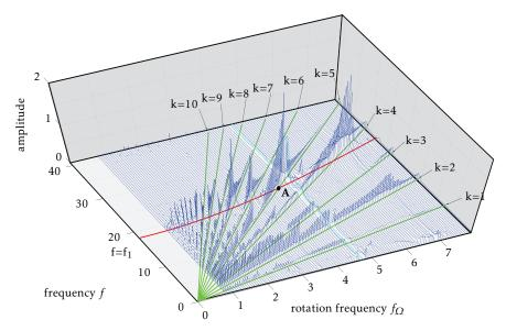
Figure 17: Spectrum of the radial displacement of the the leading edge node in configuration 2
