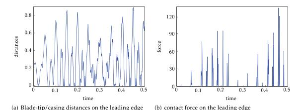
Figure 14: Blade-tip/casing contact simulation (case 1,  $\Omega = 35$ )
