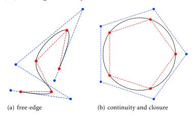
Figure 2: two types of end condition: spline (──), data points **P** (•) and control points **Q** (•)
