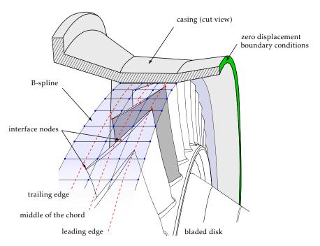
Figure 1: Surface-spline description for treatment of contact conditions between blade-tips and surrounding casing in turbomachinery
