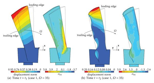
Figure 20: Displacement norm and  $\sigma_{xx}$  stress fields in one blade
