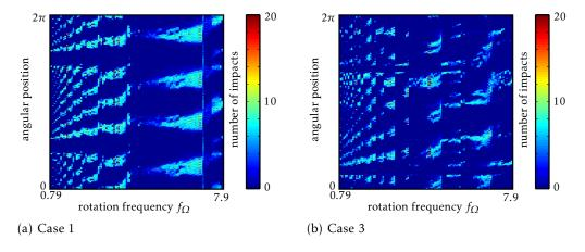
Figure 19: Contact areas between the blade leading edge and the casing over twenty revolutions
