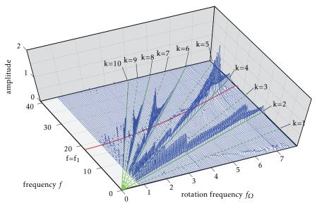
Figure 16: Spectrum of the radial displacement of the the leading edge node in configuration 1
