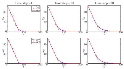
**Fig. 2** Finite element approximation (solid red line) and Reduced basis approximation (blue +) at time steps  $t/\Delta t=1$ ,  $t/\Delta t=10$  and  $t/\Delta t=T/\Delta t=20$ . The payoff function  $\psi$  is represented with the black dashed line. The reduced bases that are used have been generated by  $(\widetilde{N}_V,N_W)=(8,8)$  (plots on the top) or  $(\widetilde{N}_V,N_W)=(16,16)$  (plots on the bottom).
