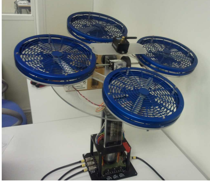
Figure 4: Quad-rotor system with a wireless Integrated Measurement Unit (IMU).
