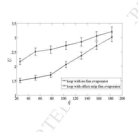
Fig. 11. Total heat transfer rate defined by equation (20)  $[kW/m^2 K]$  as a function of heat flux  $[kW/m^2]$ . Squares and triangles represent respectively the no-fins evaporator and the strip-fins evaporator.
