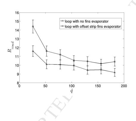
Fig. 10. Condenser thermal resistance  $R_{cond}$  [K/kW] defined by equation (19) as a function of heat flux  $\dot{q}$  [kW/m<sup>2</sup>]. Squares and triangles represent respectively the offset strip fins and no fins evaporator mounted in the loop.
