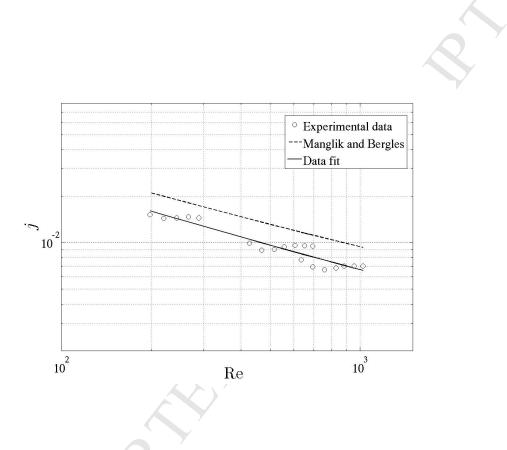
Fig. 4. Colburn factor in evaporator with offset strip fins geometry
