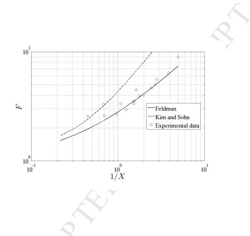
Fig. 7. Reynolds factor F obtained from experimental data (symbols) and from equations (11) (dashed line) and (12) (solid line)
