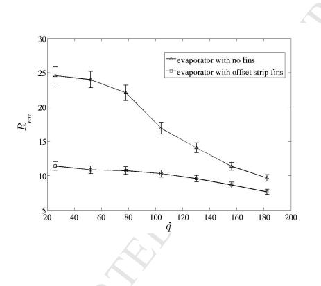
Fig. 9. Evaporator thermal resistance  $R_{ev}$  [K/kW] defined by equation (18) as a function of heat flux  $\dot{q}$  [kW/m<sup>2</sup>]. Squares and triangles represent respectively the offset strip fins and no fins evaporator.
