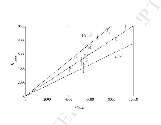
Fig. 8. Comparison of measured heat transfer coefficient with correlation (8-17)  $\rm [W/(m^2~K)]$
