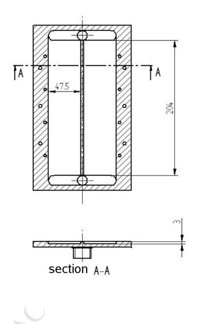
Fig. 2. Sketch of the evaporator.
