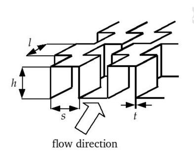
Fig. 3. Sketch of the offset strip fins geometry.
