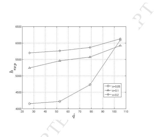
Fig. 6. Experimental boiling heat transfer coefficient  $[W/(m^2K)]$  in offset strip fins geometry as a function of heat flux  $[kW/(m^2)]$
