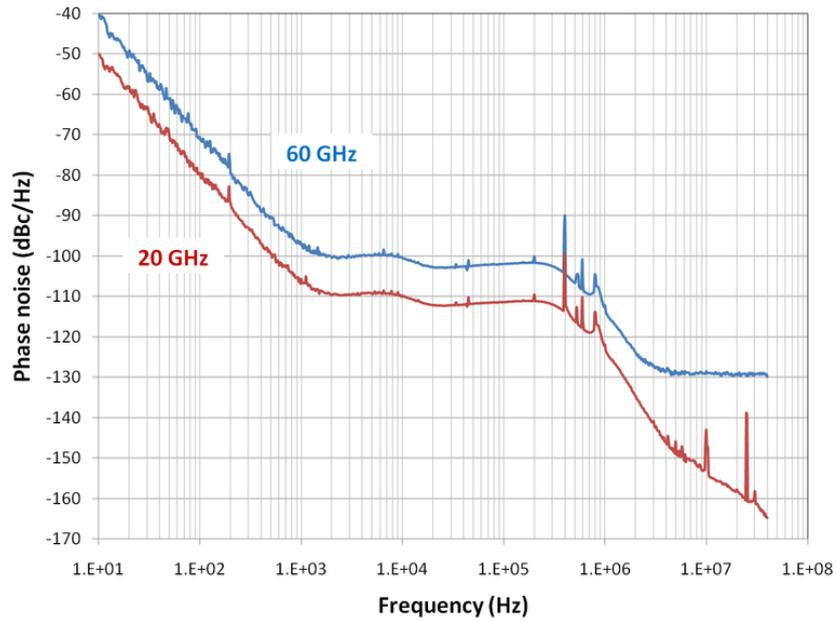
**Figure 8 :** Phase noise spectrum of the output 60 GHz signal (top curve) compared to the phase noise spectrum of the 20 GHz source (bottom curve) in case of a multiplication by 3. The two curves are perfectly parallel, with a difference of 9.5 dB corresponding to the multiplication factor. Above 3 MHz offset, the noise floor of the optical link can be observed
