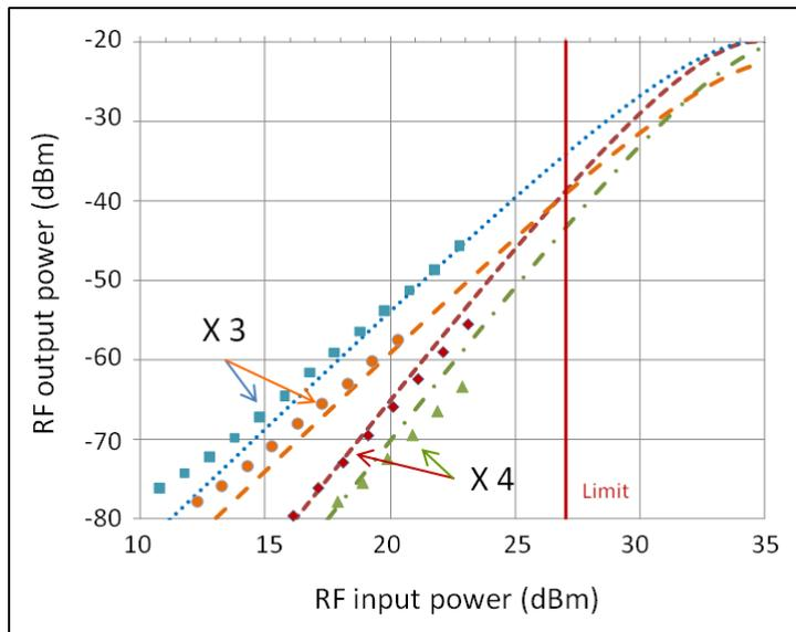
**Figure 5 :** Simulated (lines) and measured (dots) output power level at 50 GHz and 60 GHz. At low input power, the higher level is measured for a 50 GHz signal obtained from 16.66 GHz multiplied by 3, then a 60 GHz signal obtained from 20 GHz (X3), then a 50 GHz signal obtained from 12.5 GHz (X4) and finally a 60 GHz signal obtained from 15 GHz (X4).
