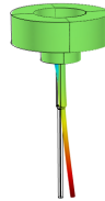
Figure 10. First eigenmode of the viscometer in the viscous fluid: the fluid domain is replaced by an impedance term.
