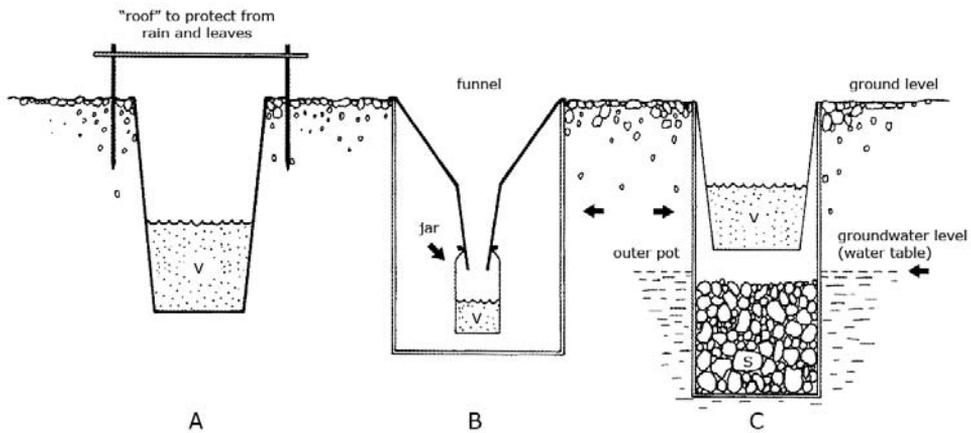
**Figure 2.** Different pitfall types. **A** = Jar or yoghurt can. **B** and **C** = traps with an outer can to make collecting of the sample easier. **B** = funnel trap with small jar. **C** = trap for moist biotopes (the outer can contains gravel or stones to prevent the can from being pushed up by groundwater). **V** = preservative (usually formaldehyde 3–4% or propylene glycol), **S** = stones or gravel.
