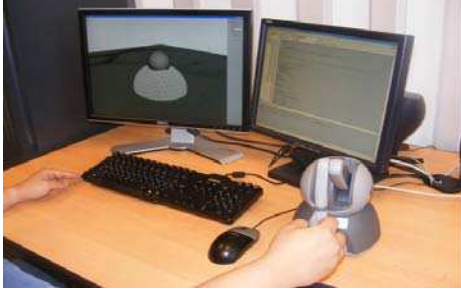
Fig. 8. Real-time indentation simulator using the Omni haptic interface.
