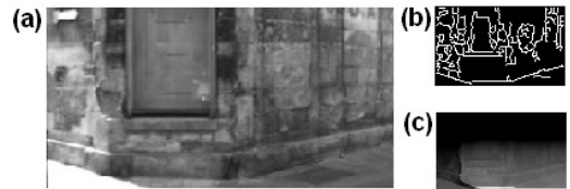
Fig. 9 – (a) Original image (in front of a wall) and its road detection result in (c); (b) Canny edge detection result.
