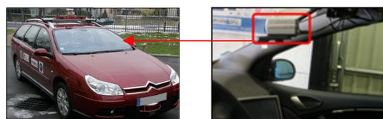
Fig. 14. Carmen: The experimental vehicle with the monocular vision system.
