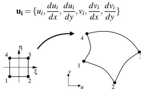
Figure 1: Hermitte element (dof and reference element)
