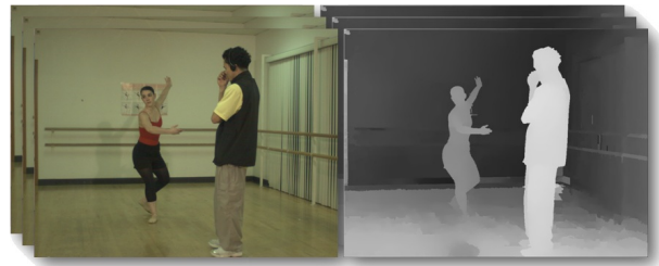
Fig. 1. MVD data consist of texture (left) and depth information (right).
