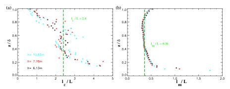
FIGURE 5 – (a) Ratio of the integral length scale and the dissipative length  $(l_{\varepsilon}/L)$  at several x positions as a function of  $z/\delta$ . (b) Ratio of the integral length scale and the dissipative length  $(l_m/L)$  at several x positions as a function of  $z/\delta$ .
