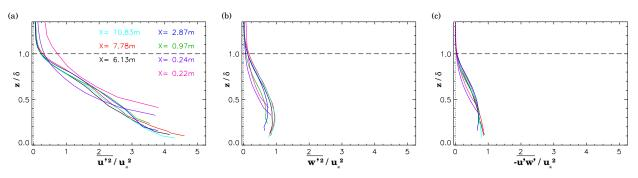
FIGURE 1 – Normalized profiles of  $\overline{u'^2}/{u_*}^2$ ,  $\overline{w'^2}/{u_*}^2$  and  $\overline{u'w'}/{u_*}^2$  (respectively (a), (b) and (c)) as a function of  $z/\delta$  for all positive measured x positions.
