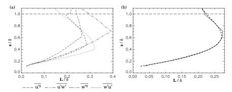
FIGURE 4 – (a): Integral length normalized by  $\delta$  for  $\overline{u'^2}$  (dashed lines),  $\overline{w'^2}$  (dash-dot lines),  $\overline{u'w'}$  (dash-dot-dot-dot-line) and  $\overline{w'u'}$  (doted lines) following the vertical direction. (b): Mean experimental integral length scale (L) (solid line) and its fit (dashed line).
