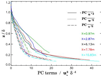
FIGURE 3 – Normalized magnitude of the pressure-correlation terms of  $\overline{u'^2}$ ,  $\overline{w'^2}$  and  $\overline{v'^2}$  as a function of  $z/\delta$  for all positive measured  $x$  positions.
