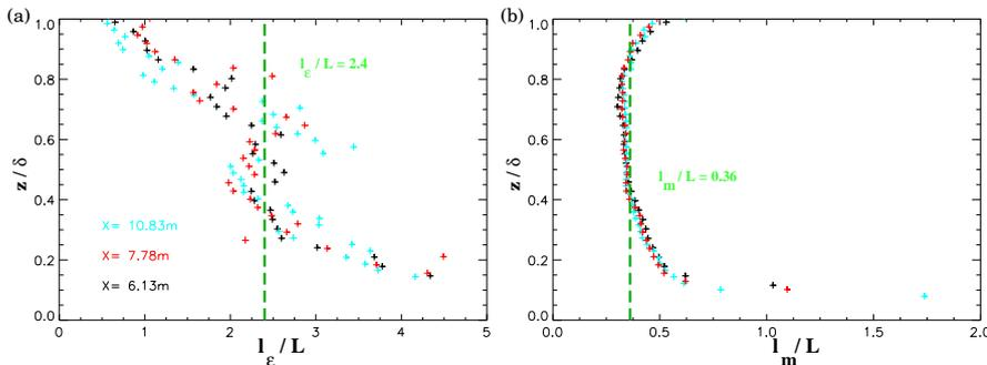
FIGURE 5 – (a) Ratio of the integral length scale and the dissipative length ( $l_\epsilon/L$ ) at several  $x$  positions as a function of  $z/\delta$ . (b) Ratio of the integral length scale and the dissipative length ( $l_m/L$ ) at several  $x$  positions as a function of  $z/\delta$ .
