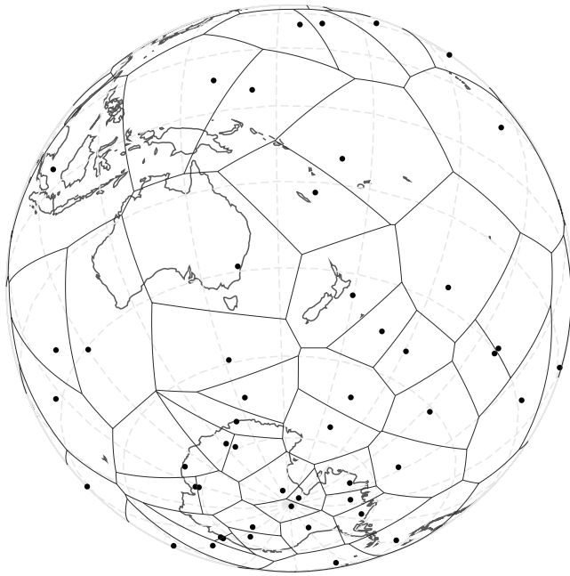
Figure 8. An example of a Voronoi diagram on the Earth's surface. The boundaries of each cell are great circles equidistant from the defining nodes, which are plotted as filled circles. Each Voronoi cell contains that part of the Earth's surface closest to the defining node. In this case the nodes are randomly positioned. The Voronoi diagram is used to build qualitative measures of model constraint in section 4.
