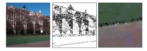
Fig. 16 Edge detection and "noise pixels" around an edge.
