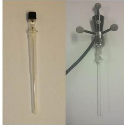
Fig. 3: Anesthetic (left) and instrumented (right) needles for position and force/torque measurement
