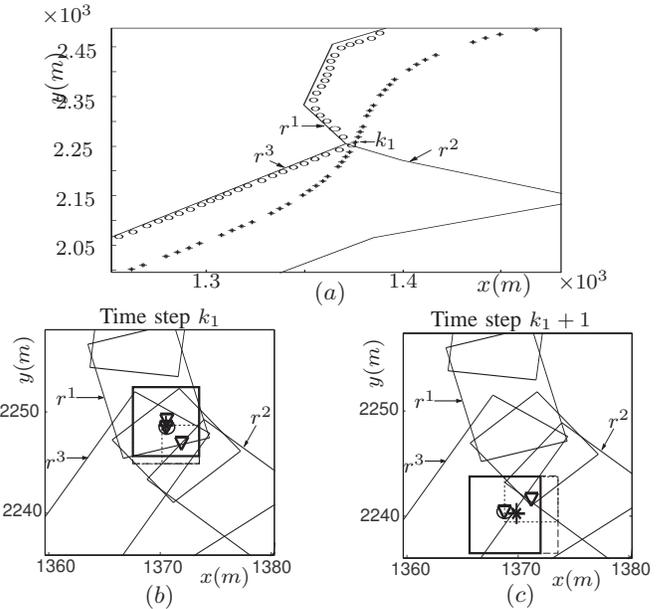
Fig. 16. Experimental results at a junction. BMM results and GPS positions are plotted as (o) and (\*) points, respectively (a). In sub-figures (b) and (c), the estimated positions on CRs, overall estimated positions and GPS measurements are represented by ( $\nabla$ ) points, (o) points and (\*) points, respectively. The dashed and bold rectangles represent the box states of CRs and the box states corresponding to the selected road, respectively.
