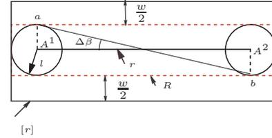
Fig. 4. Rectangular road  $[r]$  constructed using map data, geometrical errors and the road width. The road  $r$  is represented by two node points ( $A^1, A^2$ ). Two circles of radius  $l$  characterize the positional error.  $\Delta\beta$  characterizes the shape error and  $w$  is the road width.
