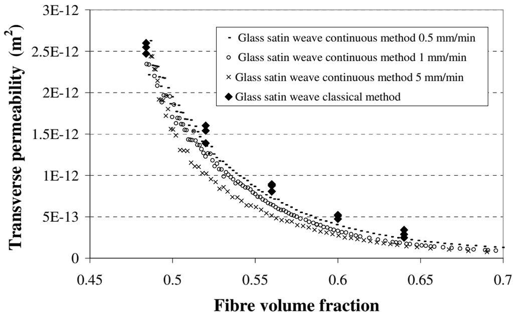
Figure 1: Continuous and “classical” transverse permeability a glass satin weave:
