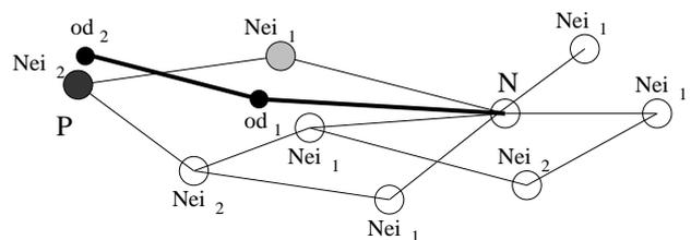
Figure 3: Illustration of the use of idiothetic data for activity updates.  $Nei_k$  is the set of all the nodes linked to node  $N$  by  $k$  connections, and  $od_k$  is the position of the robot at time  $t - k$  as measured by the odometry relatively to node  $N$ . In this example, the activity of node  $N$  will be a function of the activity of node  $P$ , at time  $t - 2$  (see text for details).
