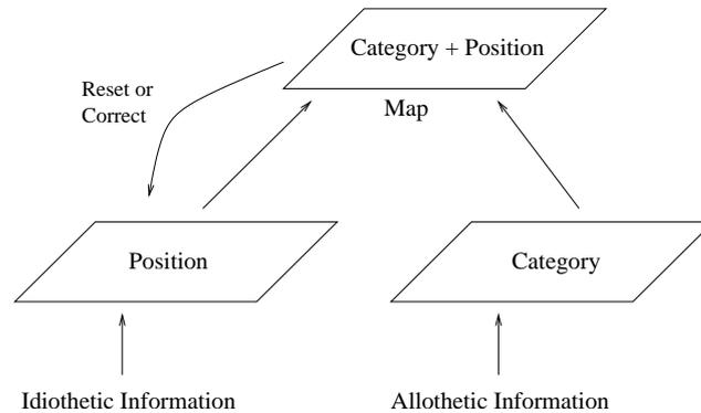
Fig. 19. A model structure that allows position tracking with a topological map and metric position estimates (see text for details).
