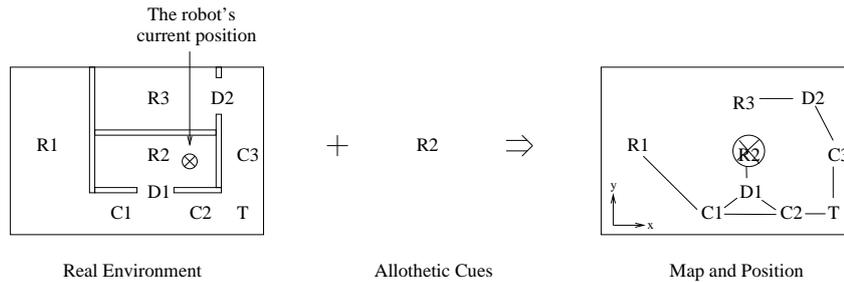
Fig. 11. When an *absolute diktiometric map*, in which each node encodes a unique sensory situation, is available, recognizing the node which corresponds to the current sensory situation allows the robot's metric position to be derived.
