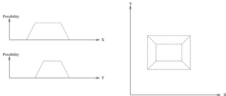
Fig. 26. Example of position representation using fuzzy sets. The left portion of the figure shows the projection of the set on the  $x$  and  $y$  axes. The right part shows the position possibility in the  $x, y$  space. The height of the fuzzy set at a given position represents the credibility for this position to be the robot's current position.
