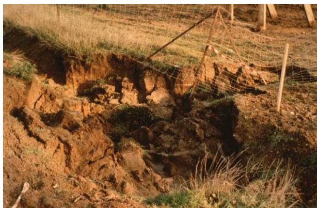
Figure 1. Collapse behaviour in shallow layers of loess directly exposed to climatic actions
