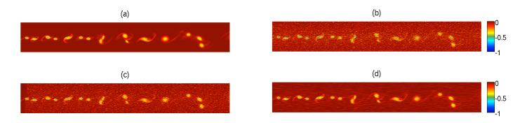
Figure 1. Vorticity fields at the end of the assimilation window. (a) True field; (b) Noisy observation; (c) Field obtained by starting from noisy observation at the begining of the assimilation window; (d) Field obtained by starting from the retrieved optimal initial conditions.
