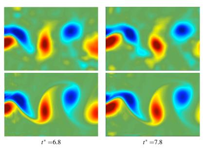
Figure 6. VDA cylinder wake experimental test *B*. Vorticity fields at two consecutive discrete instants in the assimilation window. Experimental observations (*Top*); Assimilated state (*Bottom*).
