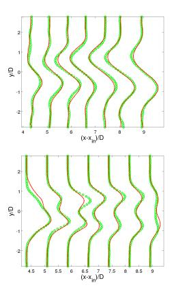
Figure 5. VDA cylinder wake experimental test *A*. Longitudinal evolution of (top) the mean vorticity and (bottom) the vorticity fluctuation  $\langle \omega' \omega' \rangle$ ; solid lines: assimilated solution; symbols: observations.
