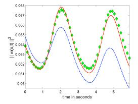
Figure 2. VDA cylinder wake twin test. Temporal evolution of the squared norm of the vorticity field; diamonds: observations; dashed line: initial approximation; solid line: assimilated solution.
