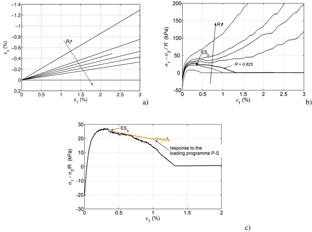
Fig. 1. a) Proportional strain loading paths applied to the sample for  $R = 0.7; 0.8; 0.825; 0.85; 0.875; 0.9; 1.0$ ; b) computed responses; c) computed response to the proportional strain path for  $R = 0.825$ , and computed response to the loading programme P-S.
