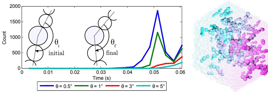
Fig. 6. (Left) The number of particles in buckling force chains which buckle by no less than the threshold value of  $\theta$ ,  $\theta_b \geq \theta$ , for one time step in the simulation. Inset illustrates the buckling angle  $\theta_b = \theta_i - \theta_f$ . (Right) Buckling force chains at simulation time of 0.0606, where  $\theta_b \geq 1.0^\circ$ : a total of 627 particles are in this set.
