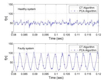
Fig. 7. FM demodulated signals for the healthy and faulty machines (bearing fault) with 300-W load.
