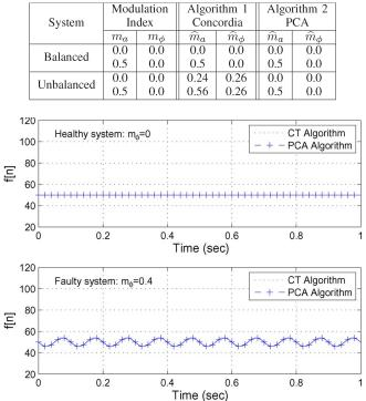
Fig. 4. FM demodulated signals for a healthy  $(m_{\phi} = 0)$  and a faulty  $(m_{\phi} = 0.4)$  balanced system.
