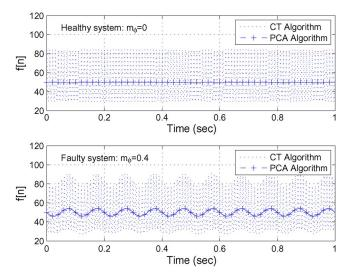
Fig. 5. FM demodulated signals for a healthy  $(m_{\phi} = 0)$  and a faulty  $(m_{\phi} = 0.4)$  unbalanced system.
