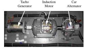
Fig. 6. Mechanical part of the experimental setup. Faulty machines are simulated with artificially deteriorated bearings [36].
