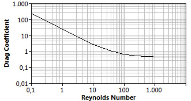
Fig. 3: Drag coefficient vs. Reynolds number, Eq. (21).
