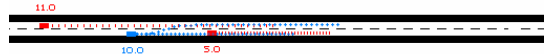
Fig. 10. Scenario for the algorithm example: overtaking of a slower vehicle by the ego vehicle
