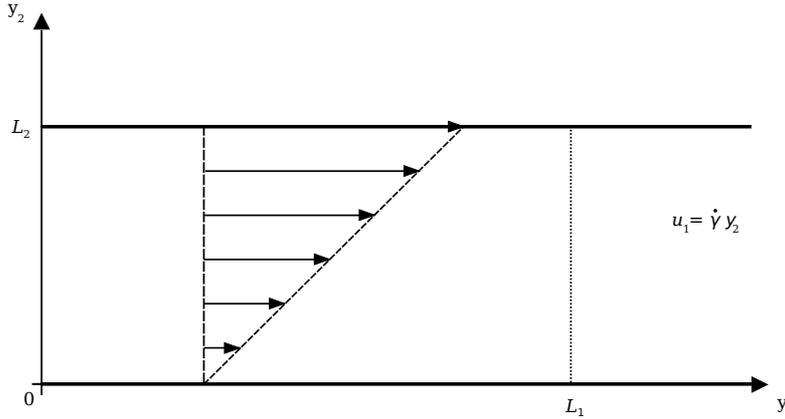
Figure 1: Shear flow: intersection with plane  $y_3 = c \in (0, L_3)$ .
