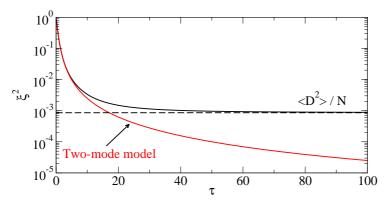
Fig. 4. (Color online) Black solid line: Squeezing parameter in the thermodynamic and weakly interacting limit (60) as a function of the renormalized time  $\tau$  (59). Parameters:  $k_B T/\rho g = 1$  and  $\sqrt{\rho a^3} = 10^{-3}$ . Black dashed line: asymptotic value (61). Red solid line: two-mode model prediction.
