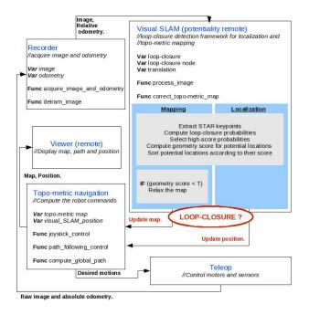
Fig. 2. Diagram of the developed system. Each box represents an uobject.
