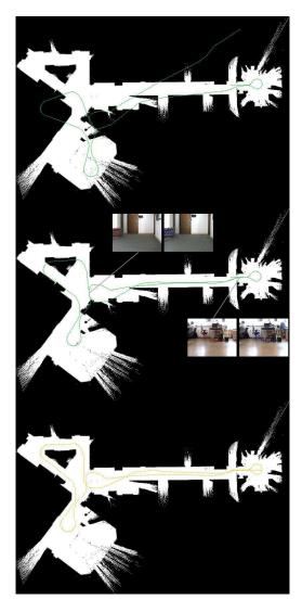
Fig. 1. Comparison of topo-metrical mapping and laser mapping. 1. Raw odometry 2. Corrected odometry applying graph relaxation taking into account the visual loop-closure (two loop-closure locations detected) 3. Ground truth trajectory (SLAM Laser). The three trajectories are shown in the frame of the reference laser map.
