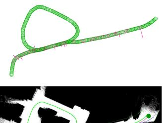
Fig. 6. Another example of the path following system illustrating the use of Dijkstra algorithm to replay a short-cut trajectory and the use of different sampling frequencies for mapping and navigation.
