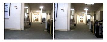
Fig. 3. Illustration of the qualitative visual localization. A loop-closure is detected between image 9 (right) and image 45 (left) with 33 pixels of x-axis translation. The computed corresponding angle of robot rotation is 4.73 degrees.
