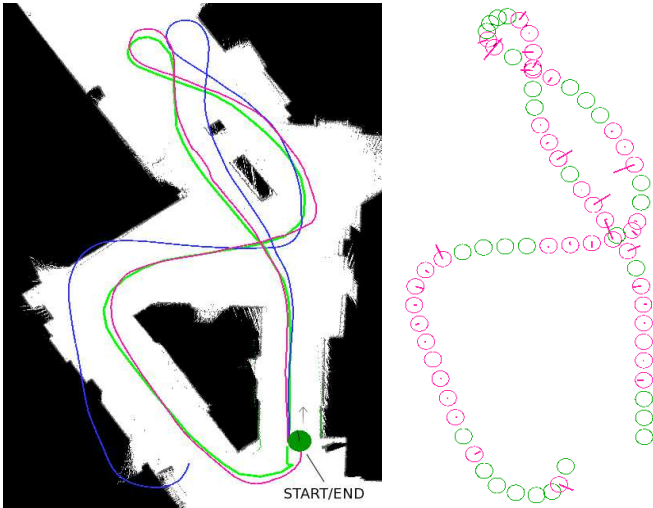
Fig. 4. Left: Example of vision-based path following replaying the trajectory used for mapping. The green and pink trajectories are the laser SLAM trajectory recorded during the mapping phase and the autonomous replay phase respectively (approx path length 30m). The blue trajectory is the odometry recorded by the robot during the replay phase. Right: Topometric map of the environment created during the same experiment. Green and pink circles are the nodes of the topological map, displayed here without map relaxation as we have not close loops during the learning phase. The pink circles are the loop-closure places detected during the replay phase. The length of line in the middle of the pink circles is proportional to the x-axis translation computed from the matching images.
